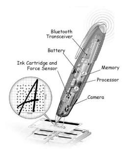
To understand the use of the pen must be instructed in its use. He reads a frame generated by an algorithm, using an infrared laser camera placed under the mine (not to confront). If the mask (by rule), the pen can no longer function.
